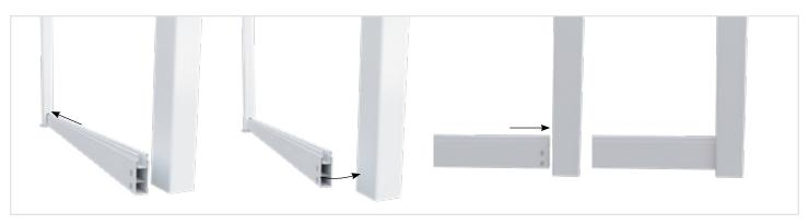
8 Slide bottom rail with aluminium insert into first post as far as possible and lever into adjacent post. Slide back bottom rail to ensure notches have passed into adjacent post.
